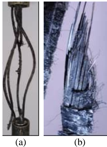
Figure 7: (a) & (b) CFCC (CFRP) strand, tensile tested to failure after 1 month exposure to acidic aggressive groundwater.
