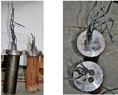
Figure 2 Failure of CFRP strand due to rupture within free length.
