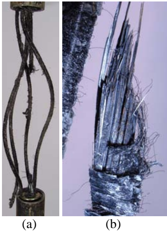
Figure 9: (a) & (b) CFCC (CFRP) strand, tensile tested to failure after 1 month exposure to acidic aggressive groundwater.
