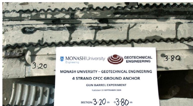
Figure 3: Dissection of 4 strand CFCC gun barrel test: location of apparent free length
